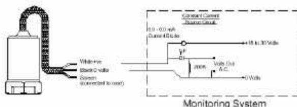
Fig 3: Constant Current Power Supply
