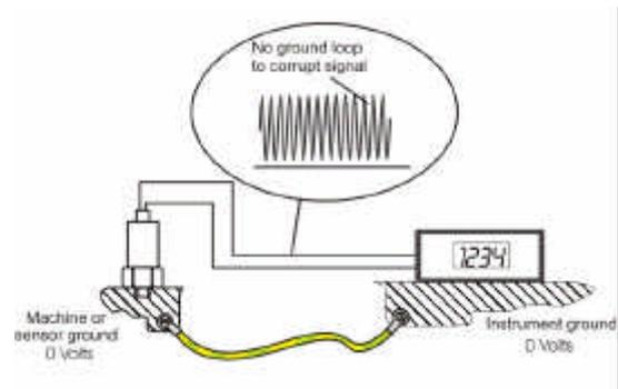
Fig 6: Eliminating ground loops
