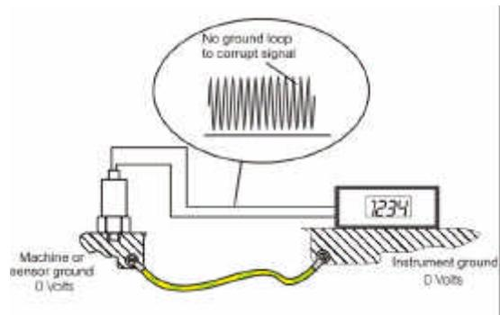
Fig 6: Eliminating ground loops
