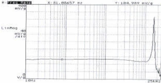
Fig 4: Typical Response Curve for MTN/1100
