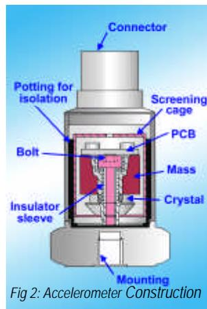
Fig 2: Accelerometer Construction
