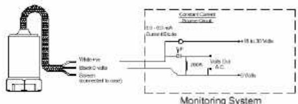
Fig 3: Constant Current Power Supply
