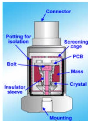
Fig 2: Accelerometer Construction
