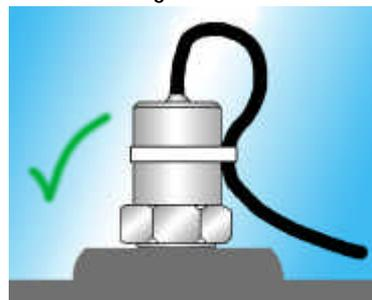
Fig 7: Removing connection strain by anchoring cable to the accelerometer body.
