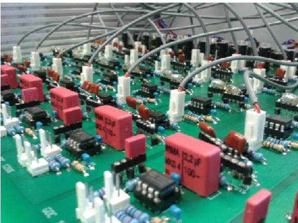
**Monitran has designed and is supplying high-accuracy signal conditioning units for interfacing with hundreds of thin film heat transfer gauges the Oxford Turbine Research Facility (OTRF) is using to investigate aero-engine turbine blade cooling techniques.**
