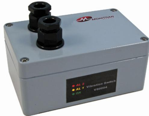
The MTVS0004 Vibration Switch offers a low cost, simple to install and operate solution to protect all sorts of rotating machinery; motors, pumps, fans, gearboxes etc. It's durable case with high IP rating is suitable for long life in harsh industrial environments. Measurements are made in velocity and compatible with ISO10816 Machine Vibration Severity Test.
