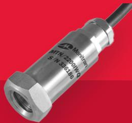
The MTN/2200TW is a submersible dual output sensor. It has an isolated AC output for measuring acceleration (100mV/g as standard, over the frequency range 2Hz to 10kHz) and an isolated DC output for measuring temperature (10mV/C).
