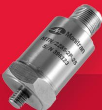
The MTN/2285-2P/4P/C is suitable for use in most industrial monitoring applications. Its output is proportional to velocity and it has a frequency range of 2Hz to 1kHz, a temperature range of -25°C to 90°C and is sealed to IP67.
