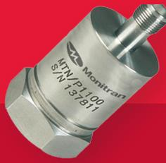
The MTN/P1100\* is a high sensitivity (1100pC/g @ 80Hz) accelerometer. It has frequency range of 1Hz to 10kHz and a temperature range of -55°C to 250°C.
