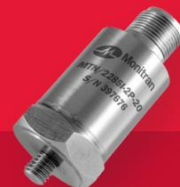
The MTN/2285I is an ATEX and IECEx Group II certified, intrinsically safe accelerometer. It is sealed to IP67, has a frequency range of 2Hz to 1kHz and a temperature range of -25°C to 90°C. A variant is also available for mining applications.
