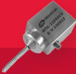
The MTN/1105SCE\* is constant current AC output accelerometer for vibration analysis at temperatures up to 250°C. It has a frequency range of 1Hz to 10kHz and a sensitivity of 100mV/g (others are available upon request).
