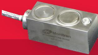
2285STC/532 General purpose, side-entry velocity transducer with dual independent 4-20mA outputs. Sealed to IP65 with 4-20mA outputs proportional to velocity and temperature range that can connect directly to PLC, DCS and other industrial controllers. Frequency range 2Hz to 1kHz.
