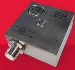
MTN/2330 Heavy-duty constant current accelerometer with 3 isolated 100mV/g AC outputs (X, Y and Z axes). Ideal for any application where vibration in all three spatial axes needs to be measured. Frequency range 2Hz to 10kHz. Temperature version also available.
