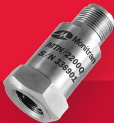
The MTN/2200-2P/4P/C is suitable for use in most industrial applications. It has a frequency range of 2Hz to 10kHz, a temperature range of -55°C to 140°C and is sealed to IP67.
