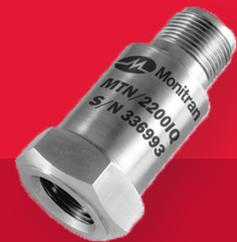
The MTN/2200I is an ATEX and IECEx Group II certified, intrinsically safe sensor, it has a frequency range of 2Hz to 10kHz and a temperature range of -55°C to 90°C.
